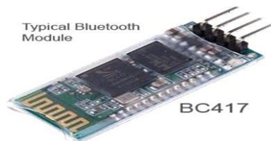
Fig 4. Bluetooth module BC417
